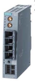
SCALANCE M876-3 3G router; for the wireless IP communication of Ethernet-based Programmable controllers via 3G mobile radio HSPA+/EV-DO, VPN, Firewall, NAT 4-port switch; Antenna diversity; 1x digital input, 1x digital output; observe national approvals! Observe provider's approvals!
