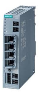
SCALANCE M826-2 SHDSL router; for the IP communication via 2-wire and 4-wire cables from Ethernet-based Programmable controllers; SHDSL topology: Point-to-point, bonding, line bridge mode; Routing mode with VPN, Firewall, NAT; 4-port switch; 1x digital input, 1x digital output
