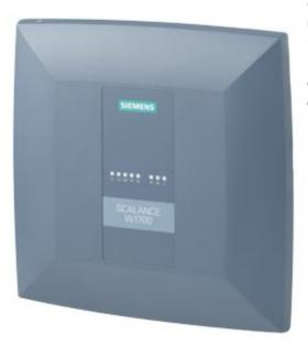
IWLAN access point, SCALANCE W1788-2IA M12, 2 radios, 8 internal antennas, iFeatures support via CLP, IEEE 802.11a/b/g/h/n/ac, 2.4/5 GHz, gross 1733 Mbit/s per radio, 2x M12 max. 1 Gbit/s, PoE, redundant 24 V DC, M12 A-coded IP65, -20..+70 °C, CLP slot, WPA2/802.11i/e, observe national approvals! CERT ID: RAPAC-W2-M12-I4, includes: MPCIE-R1-ABGNAC-U4 Scope of delivery: Manuals on DVD, German/English, 1x terminal block; for operation outside of USA/Israel
