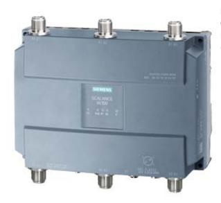
IWLAN Access Point, SCALANCE W788-2 M12 EEC USA, 2 radios, 6 N-CON antenna port, iFeatures support via key plug, IEEE 802.11a/b/g/h/n, 2.4/5GHz, gross 450 Mbit/s per radio, 1x M12 max. 1 Gbit/s, PoE, redundant 24 V DC, M12 A-coded IP65, -40...+70 °C, plug slot WPA2/802.11i/e,conformal coating EN 50155, EN 45545, observe national approvals! CERT ID: RAPN-W2-M12-E3, includes: MPCIE-R1-ABGN-U3, scope of delivery: Manuals on CD-ROM, German/English, M12 sealing caps, only for operation in USA
