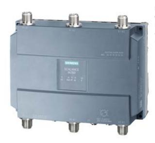
IWLAN Access Point, SCALANCE W788-2 M12 EEC, 2 radios, 6 N-CON antenna port, iFeatures support via key plug, IEEE 802.11a/b/g/h/n, 2.4/5GHz, gross 450 Mbit/s per radio, 1x M12 max. 1 Gbit/s, PoE, redundant 24 V DC,M12 A-coded IP65, -40..+70 °C, plug slot, WPA2/802.11i/e,conformal coating EN 50155, EN 45545, observe national approvals! CERT ID: RAPN-W2-M12-E3, includes: MPCIE-R1-ABGN-U3, scope of delivery: Manuals on CD-ROM, German/English, M12 sealing caps, for operation outside of USA/Israel
