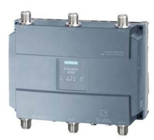
IWLAN Access Point, SCALANCE W788-2 M12, 2 radios, 6 N-CON antenna port, iFeatures support via key plug, IEEE 802.11a/b/g/h/n, 2.4/5GHz, gross 450 Mbit/s per radio, 1x M12 max. 1 Gbit/s, PoE, redundant 24 V DC,M12 A-coded IP65, -20..+60 °C, plug slot, WPA2/802.11i/e, observe national approvals! CERT ID: RAPN-W2-M12-E3, includes: MPCIE-R1-ABGN-U3, scope of delivery: Manuals on CD-ROM, German/English, M12 sealing caps, only for operation in USA
