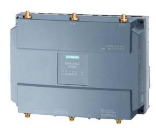
IWLAN Access Point, SCALANCE W788-2 RJ45, 2 radios, 6 R-SMA antenna port, iFeatures support via key plug, IEEE 802.11a/b/g/h/n, 2.4/5GHz, gross 450 Mbit/s per radio, 1x RJ45 max. 1 Gbit/s, PoE, redundant 24 V DC, terminal block, IP30, -20..+60 °C, plug slot, WPA2/802.11i/e, Signaling contact observe national approvals! CERT ID: RAPN-W2-RJ-E3, includes: MPCIE-R1-ABGN-U3, scope of delivery: Manuals on CD-ROM, German/English, 2x terminal blocks; only for operation in USA
