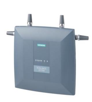
IWLAN access point, SCALANCE W1788-1 M12, 1 radio, 4 N-CON antenna port, iFeatures support via CLP, IEEE 802.11a/b/g/h/n/ac, 2.4/5 GHz, gross 1733 Mbit/s per radio, 2x M12 max. 1 Gbit/s, PoE, redundant 24 V DC,M12 A-coded IP65, -20..+70 °C, CLP slot, WPA2/802.11i/e, observe national approvals! CERT ID: RAPAC-W1-M12-E4, includes: MPCIE-R1-ABGNAC-U4 Scope of delivery: Manuals on DVD, German/English, M12 sealing caps, for operation outside of USA/Israel
