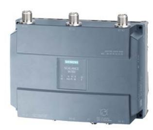
IWLAN Access Point, SCALANCE W788-1 M12, 1 radio, 3 N-CON antenna port, iFeatures support via key plug, IEEE 802.11a/b/g/h/n, 2.4/5GHz, gross 450 Mbit/s per radio, 1x M12 max. 1 Gbit/s, PoE, redundant 24 V DC,M12 A-coded IP65, -20..+60 °C, plug slot, WPA2/802.11i/e, observe national approvals! CERT ID: RAPN-W1-M12-E3, includes: MPCIE-R1-ABGN-U3, scope of delivery: Manuals on CD-ROM, German/English, M12 sealing caps, only for operation in USA
