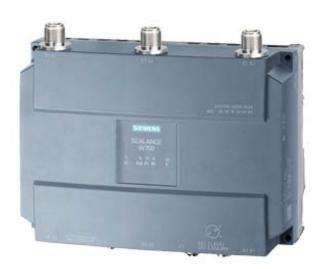
IWLAN Access Point, SCALANCE W788-1 M12, 1 radio, 3 N-CON antenna port, iFeatures support via key plug, IEEE 802.11a/b/g/h/n, 2.4/5GHz, gross 450 Mbit/s per radio, 1x M12 max. 1 Gbit/s, PoE, redundant 24 V DC,M12 A-coded IP65, -20..+60 °C, plug slot, WPA2/802.11i/e, observe national approvals! CERT ID: RAPN-W1-M12-E3, includes: MPCIE-R1-ABGN-U3, scope of delivery: Manuals on CD-ROM, German/English, M12 sealing caps, for operation outside of USA/Israel
