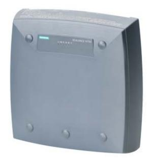
IWLAN Access Point, SCALANCE W786-2 RJ45, 2 radios, 6 R-SMA antenna port, iFeatures support via key plug, IEEE 802.11a/b/g/h/n, 2.4/5GHz, gross 450 Mbit/s per radio, 1x RJ45 max. 1 Gbit/s, PoE, redundant 24 V DC, terminal block, 110 - 230 V AC via PS791-2AC IP65, -40..+60 °C, plug slot, WPA2/802.11i/e, observe national approvals! CERT ID: EAPN-W2-RJ-E3, includes: MPCIE-R1-ABGN-U3, scope of delivery: Manuals on CD-ROM, German/English, 1x terminal block; for operation in the USA
