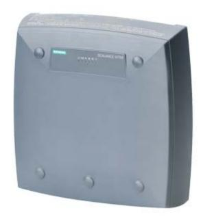
IWLAN Access Point, SCALANCE W786-2 RJ45, 2 radios, 6 R-SMA antenna port, iFeatures support via key plug, IEEE 802.11a/b/g/h/n, 2.4/5GHz, gross 450 Mbit/s per radio, 1x RJ45 max. 1 Gbit/s, PoE, redundant 24 V DC, terminal block, 110 - 230 V AC via PS791-2AC IP65, -40..+60 °C, plug slot, WPA2/802.11i/e, observe national approvals! CERT ID: EAPN-W2-RJ-E3, includes: MPCIE-R1-ABGN-U3, scope of delivery: Manuals on CD-ROM, German/English, 1x terminal block; for operation outside of USA/Israel
