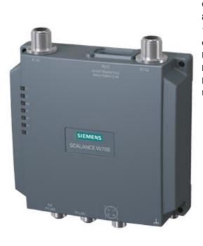
IWLAN access point, SCALANCE W778-1 M12 EEC, 1 radio, 2 N-CON antenna port, iFeatures support via key plug, IEEE 802.11a/b/g/h/n, 2.4/5 GHz, gross data rate 300 Mbit/s, 2x M12 max. 100 Mbit/s, PoE integrated 2-port switch, redundant 24 V DC, M12 Acoded IP65, -30... 70 °C, plug slot WPA2/802.11i/e,conformal coating EN 50155, EN 45545, observe national approvals! CERT ID: MSN65-W1-M12-E2 Scope of delivery: Manuals on CD-ROM, English/German; M12 sealing caps, for operation outside of USA/Israel
