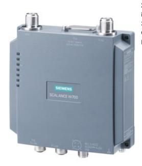
IWLAN access point, SCALANCE W778-1 M12, 1 radio, 2 N-CON antenna port, iFeatures support via key plug, IEEE 802.11a/b/g/h/n, 2.4/5 GHz, gross data rate 300 Mbit/s, 2x M12 max. 100 Mbit/s, PoE integrated 2-port switch, redundant 24 V DC, M12 A-coded IP65, - 30... 65 °C, plug slot WPA2/802.11i/e, observe national approvals! CERT ID: MSN65-W1-M12-E2 Scope of delivery: Manuals on CD-ROM, English/German; M12 sealing caps, for operation in the USA
