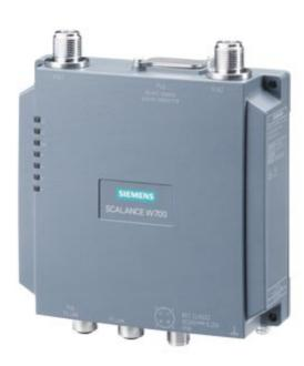
IWLAN access point, SCALANCE W778-1 M12, 1 radio, 2 N-CON antenna port, iFeatures support via key plug, IEEE 802.11a/b/g/h/n, 2.4/5 GHz, gross data rate 300 Mbit/s, 2x M12 max. 100 Mbit/s, PoE integrated 2-port switch, redundant 24 V DC, M12 A-coded IP65, - 20... 60 °C, plug slot WPA2/802.11i/e, observe national approvals! CERT ID: MSN65-W1-M12-E2 Scope of delivery: Manuals on CD-ROM, English/German; M12 sealing caps, for operation outside of USA/Israel
