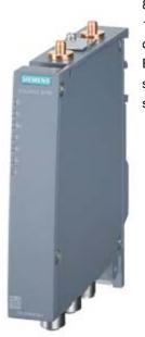
IWLAN Access Point, SCALANCE W774-1 M12 EEC, 1 radio, 2 R-SMA antenna port, iFeatures support via key plug, IEEE 802.11a/b/g/h/n, 2.4/5GHz, gross data rate 300 Mbit/s, 2x M12 max. 100 Mbit/s, PoE integrated 2-port switch, redundant 24 V DC,M12 Acoded IP30, -30... 65 °C, plug slot WPA2/802.11i/e,conformal coating EN 50155, observe national approvals! CERT ID: MSN-W1-M12-E2, scope of delivery: Manuals on CD-ROM, English/German; M12 sealing caps, for operation in the USA
