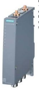
IWLAN Access Point, SCALANCE W774-1 M12 EEC, 1 radio, 2 R-SMA antenna port, iFeatures support via key plug, IEEE 802.11a/b/g/h/n, 2.4/5GHz, gross data rate 300 Mbit/s, 2x M12 max. 100 Mbit/s, PoE integrated 2-port switch, redundant 24 V DC,M12 Acoded IP30, -30... 65 °C, plug slot WPA2/802.11i/e,conformal coating EN 50155, observe national approvals! CERT ID: MSN-W1-M12-E2, scope of delivery: Manuals on CD-ROM, English/German; M12 sealing caps, for operation outside of USA/Israel
