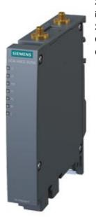
IWLAN Access Point, SCALANCE W774-1 RJ45, 1 radio, 2 R-SMA antenna port, iFeatures support via key plug, IEEE 802.11a/b/g/h/n, 2.4/5GHz, gross data rate 300 Mbit/s, 2x RJ45 max. 100 Mbit/s, PoE integrated 2-port switch, redundant 24 V DC, terminal block, IP30, -20... 60 °C, plug slot WPA2/802.11i/e, observe national approvals! CERT ID: MSN-W1-RJ-E2, scope of delivery: Manuals on CD-ROM, German/English, 1x terminal block; for operation in Israel
