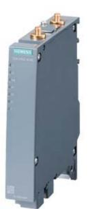
IWLAN Access Point, SCALANCE W774-1 RJ45, 1 radio, 2 R-SMA antenna port, iFeatures support via key plug, IEEE 802.11a/b/g/h/n, 2.4/5GHz, gross data rate 300 Mbit/s, 2x RJ45 max. 100 Mbit/s, PoE integrated 2-port switch, redundant 24 V DC, terminal block, IP30, -20... 60 °C, plug slot WPA2/802.11i/e, observe national approvals! CERT ID: MSN-W1-RJ-E2, scope of delivery: Manuals on CD-ROM, German/English, 1x terminal block; for operation outside of USA/Israel
