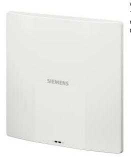
WLAN access point, SCALANCE W1750D-2IA RJ45, 2 radios, controller operation without WLC, internal antennas, IEEE802.11ac wave2 AP, MU-MIMO, gross up to 800 Mbit/s (2.4 GHz) Gross up to 1.7 Gbit/s (5 GHz), 2 x RJ45, PoE, USB, 0 °C to +50 °C, Observe national approval! Cert ID includes: MPCIE Scope of delivery: DVD, Quick Start Guide (en) manuals Ceiling bracket Type: US
