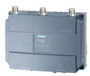
IWLAN client, SCALANCE W748-1 M12, 1 radio, 3 N-CON antenna port, iFeatures support via key plug, IEEE 802.11a/b/g/h/n, 2.4/5GHz, gross 450 Mbit/s per radio, 1x M12 max. 1 Gbit/s, PoE, redundant 24 V DC,M12 A-coded IP65, -20..+60 °C, plug slot, WPA2/802.11i/e, Signaling contact observe national approvals! CERT ID: RAPN-W1-M12-E3, includes: MPCIE-R1-ABGN-U3, scope of delivery: Manuals on CD-ROM, English/German; M12 sealing caps, for operation in the USA
