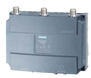
IWLAN client, SCALANCE W748-1 M12, 1 radio, 3 N-CON antenna port, iFeatures support via key plug, IEEE 802.11a/b/g/h/n, 2.4/5GHz, gross 450 Mbit/s per radio, 1x M12 max. 1 Gbit/s, PoE, redundant 24 V DC,M12 A-coded IP65, -20..+60 °C, plug slot, WPA2/802.11i/e, Signaling contact observe national approvals! CERT ID: RAPN-W1-M12-E3, includes: MPCIE-R1-ABGN-U3, scope of delivery: Manuals on CD-ROM, English/German; M12 sealing caps, for operation outside of USA/Israel
