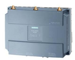
IWLAN client, SCALANCE W748-1 RJ45, 1 radio, 3 R-SMA antenna port, iFeatures support via key plug, IEEE 802.11a/b/g/h/n, 2.4/5GHz, gross 450 Mbit/s per radio, 1x RJ45 max. 1 Gbit/s, PoE, redundant 24 V DC, terminal block, IP30, Temp: -20 ...+60 °C, WPA2/802.11i/e, Signaling contact observe national approvals! CERT ID: RAPN-W1-RJ-E3, includes: MPCIE-R1-ABGN-U3, scope of delivery: Manuals on CD-ROM, German/English, 2x terminal blocks; for operation in the USA
