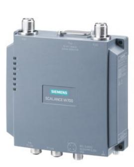
IWLAN client, SCALANCE W738-1 M12, 1 radio, 2 N-CON antenna port, iFeatures support via key plug, IEEE 802.11a/b/g/h/n, 2.4/5 GHz, gross data rate 300 Mbit/s, 2x M12 max. 100 Mbit/s, PoE integrated 2-port switch, redundant 24 V DC,M12 A-coded IP65, -20... 60 °C, plug slot WPA2/802.11i/e, observe national approvals! CERT ID: MSN65-W1-M12-E2 Scope of delivery: Manuals on CD-ROM, English/German; M12 sealing caps, for operation in the USA
