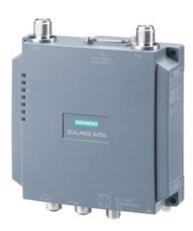
IWLAN client, SCALANCE W738-1 M12, 1 radio, 2 N-CON antenna port, iFeatures support via key plug, IEEE 802.11a/b/g/h/n, 2.4/5 GHz, gross data rate 300 Mbit/s, 2x M12 max. 100 Mbit/s, PoE integrated 2-port switch, redundant 24 V DC,M12 A-coded IP65, - 20... 60 °C, plug slot WPA2/802.11i/e, observe national approvals! CERT ID: MSN65-W1-M12-E2 Scope of delivery: Manuals on CD-ROM, English/German; M12 sealing caps, for operation outside of USA/Israel
