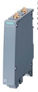
IWLAN client, SCALANCE W734-1, RJ45, 1 radio, 2 R-SMA antenna port, iFeatures support via key plug, IEEE 802.11a/b/g/h/n, 2.4/5GHz, gross data rate 300 Mbit/s, 2x RJ45 max. 100 Mbit/s, PoE integrated 2-port switch, redundant 24 V DC, terminal block, IP30, - 20... 60 °C, plug slot WPA2/802.11i/e, observe national approvals! CERT ID: MSN-W1-RJ-E2, scope of delivery: Manuals on CD-ROM, German/English, 1x terminal block; for operation outside of USA/Israel
