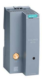
IWLAN client, SCALANCE W722-1, RJ45, 1 radio, 1 R-SMA antenna port, iFeatures support IEEE 802.11a/b/g/h/n, 2.4/5 GHz, gross data rate 150 Mbit/s, 1x RJ45 max. 100 Mbit/s, 24 V DC, terminal block, IP20, 0... +55°C, WPA2/802.11i/e, observe national approvals! CERT ID: ELN-W1-RJ-E1, scope of delivery: Manuals on CD-ROM, German/English, 1x terminal block; only for operation in Israel
