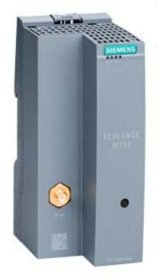
IWLAN client, SCALANCE W722-1, RJ45, 1 radio, 1 R-SMA antenna port, iFeatures support IEEE 802.11a/b/g/h/n, 2.4/5 GHz, gross data rate 150 Mbit/s, 1x RJ45 max. 100 Mbit/s, 24 V DC, terminal block, IP20, 0... +55°C, WPA2/802.11i/e, observe national approvals! CERT ID: ELN-W1-RJ-E1, scope of delivery: Manuals on CD-ROM, German/English, 1x terminal block; for operation outside of USA/Israel
