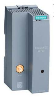
IWLAN client, SCALANCE W721-1, RJ45, 1 radio, 1 R-SMA antenna port, IEEE 802.11a/b/g/h/n, 2.4/5 GHz, gross data rate 150 Mbit/s, 1x RJ45 max. 100 Mbit/s, 24 V DC, terminal block, IP20, 0... +55°C, WPA2/802.11i/e, observe national approvals! CERT ID: ELN-W1-RJ-E1, scope of delivery: Manuals on CD-ROM, German/English, 1x terminal block; only for operation in USA
