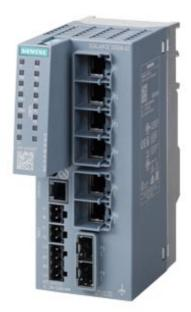
SCALANCE SC636-2C Industrial Security Appliance; For protection of devices and networks in discrete manufacturing and the process industry For protection of industrial communication with firewall; Further functions: Address translation (NAT/NAPT); Connection to SINEMA RC; 4x ports electrical 10/100/1000 Mbps RJ45 and 2x combo port electrical or optical; 10/100/1000 Mbps RJ45 or 100 Mbps SFP or 1000 Mbps SFP
