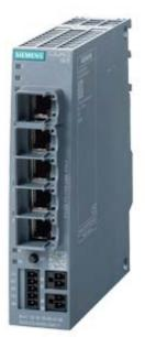
SCALANCE S615 LAN router; for protection of devices/networks in automation technology and for protection of industrial communication by means of VPN and firewall; Further functions: address conversion (NAT/NAPT), connection to SINEMA RC, 5-port switch, 1x dig. input, 1x digital output
