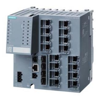
SCALANCE XM416-4C; managed modular IE switch; 16x 10/100/1000 Mbit/s RJ45; 4x 100/1000 Mbit/s SFP; contains 4 combo ports; in total 16 ports can be used; expandable to 24 ports electrical or optical; assembly: DIN rail/S7 mounting rail, PROFINET IO device; redundancy functions; office features (RSTP, VLAN, IGMP,..); C-plug in scope of delivery; Layer 3 with key plug available
