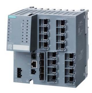
SCALANCE XM416-4C; managed modular IE switch; 16x 10/100/1000 Mbit/s RJ45; 4x 100/1000 Mbit/s SFP; contains 4 combo ports; in total 16 ports can be used; expandable to 24 ports electrical or optical; assembly: DIN rail/S7 mounting rail, PROFINET IO device; redundancy functions; office features (RSTP, VLAN, IGMP,..); C-plug in scope of delivery; Layer 3 integrated;
