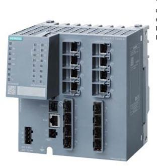
SCALANCE XM408-8C; managed modular IE switch; 8x 10/100/1000 Mbit/s RJ45; 8x 100/1000 Mbit/s SFP; contains 8 combo ports; in total 8 ports can be used; expandable to 24 ports electrical or optical; assembly: DIN rail/S7 mounting rail, PROFINET IO device; redundancy functions; office features (RSTP, VLAN, IGMP,..); C-plug in scope of delivery; Layer 3 integrated
