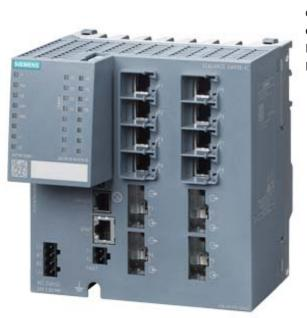
SCALANCE XM408-4C; managed modular IE switch; 8x 10/100/1000 Mbit/s RJ45; 4x 100/1000 Mbit/s ST-/SC- Pluggable as combo ports; in total 8 ports can be used; expandable to 24 ports electrical or optical; assembly: DIN rail/S7 mounting rail, PROFINET IO device; redundancy functions; office features (RSTP, VLAN, IGMP,..); C-plug in scope of delivery; Layer 3 with key plug available
