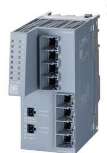
PE408PoE Port Extender for SCALANCE XM-400 managed modular IE switch; extension by 8x 10/100/1000 Mbit/s RJ45 with up to 8 ports PoE according to IEEE802.3AT; for PoE separate power supply required
