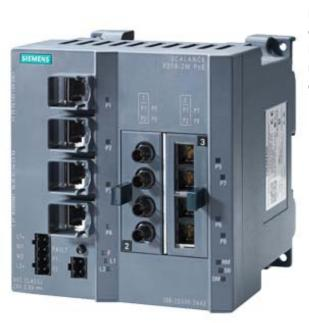
SCALANCE X308-2M PoE; managed IE switch, compact; 4x 10/100/1000 Mbit/s for RJ45 ports electrical with PoE; 2x 100/1000 Mbit/s for 2-port media modules, electrical or optical; LED diagnostics, error signaling Contact with select/set button, PROFINET IO device, network management, Integrated redundancy manager, office features (RSTP, VLAN, IGMP,...) C-plug in scope of delivery
