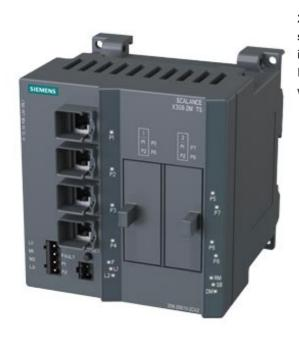
SCALANCE X308-2M TS; managed IE switch, compact; 4x 10/100/1000 Mbit/s for RJ45 ports electrical; 2x 100/1000 Mbit/s for 2-port media modules, electrical or optical; LED diagnostics; error signaling Contact; PROFINET IO device; network management; integrated redundancy manager; Office features (RSTP, VLAN, IGMP,..); C-plug in scope of delivery extended temperature range with railway approval EN 50155;
