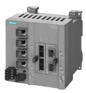
SCALANCE X308-2M; managed IE switch, compact; 4x 10/100/1000 Mbit/s for RJ45 ports electrical; 2x 100/1000 Mbit/s for 2-port media modules, electrical or optical; LED diagnostics; error signaling Contact; Select/set button; PROFINET IO device; network management; Integrated redundancy manager; office features (RSTP, VLAN, IGMP,...); C-plug in scope of delivery
