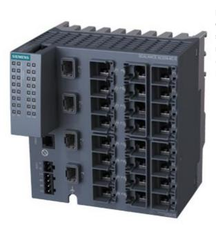
SCALANCE XC224-4C G (E/IP) manageable layer 2 IE Switch; Full Gigabit; 20x 10/100/1000 Mbps RJ45 ports; 4x 1000 Mbps combo ports (either 1000 Mbps s SFPs or 10/100/1000 Mbps RJ45 ports can be used); 1x console port; Diagnostic LED; redundant power supply; Temp. range -40 °C to +70 °C; Mounting: Standard mounting rail/S7 mounting rail/wall; redundancy functions; office features (RSTP, VLAN ,...); PROFINET IO Device; Ethernet/IP conformity; C-PLUG shaft; Default EtherNet/IP
