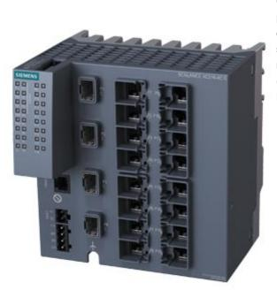
SCALANCE XC216-4C G (E/IP) manageable layer 2 IE Switch; Full Gigabit; 12x 10/100/1000 Mbps RJ45 ports; 4x 1000 Mbps combo ports (either 1000 Mbps s SFPs or 10/100/1000 Mbps RJ45 ports can be used); 1x console port; Diagnostic LED; redundant power supply; Temp. range -40 °C to +70 °C; Mounting: Standard mounting rail/S7 mounting rail/wall; redundancy functions; office features (RSTP, VLAN ,...); PROFINET IO Device; Ethernet/IP conformity; C-PLUG shaft; Default EtherNet/IP
