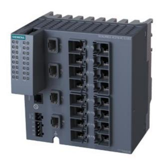
SCALANCE XC216-4C G EEC manageable layer 2 IE Switch; Full Gigabit; 12x 10/100/1000 Mbps RJ45 ports; 4x 1000 Mbps combo ports (either 1000 Mbps s SFPs or 10/100/1000 Mbps RJ45 ports can be used); 1x console port; Diagnostic LED; redundant power supply; with coated PCBs; NAMUR NE21-compliant; Temp. range - 40 °C to +70 °C; Mounting: Standard mounting rail/S7 mounting rail/wall; redundancy functions; office features (RSTP, VLAN ,...); PROFINET IO Device; Ethernet/IP conformity; C-PLUG shaft;
