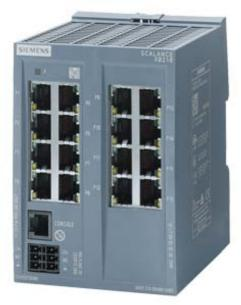
Preset for Ethernet/IP mode! SCALANCE XB216 managed Layer 2 IE Switch, 16X 10/100 Mbit/s RJ45 ports, 1x console port, Diagnostics LEDs Redundant power supply; temp. range 0 to +60 °C mounting onto standard rail; Default EtherNet/IP
