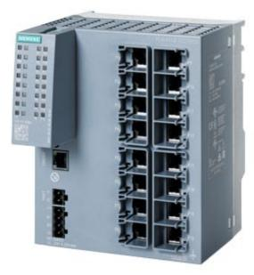
SCALANCE XC216EEC Manageable layer 2 IE switch; 16x 10/100 Mbit/s RJ45 ports; 1x console port; Diagnostics LED; Redundant power supply; with painted printed circuit boards; NAMUR NE21-compliant; Temp. range -40 °C to +70 °C Mounting: Standard mounting rail/S7 mounting rail/wall; Redundancy functions; Office features (RSTP, VLAN,...); PROFINET IO device; Ethernet/IP-compliant; C-PLUG slot;
