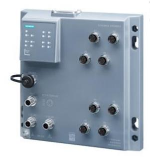
SCALANCE XP208EEC, managed IE switch with railway approval (EN 50155, EN 45545); 8x 10/100 Mbps M12 ports, IP65, LED diagnostics, error signaling contact, Redundant power supply, PROFINET IO device, network management, operable in redundant ring, Dust caps, incl. electronic Manual on CD-ROM, C-plug optional
