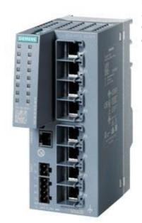
SCALANCE XC208G (E/IP) Manageable layer 2 IE switch; 8x 10/100/1000 Mbit/s RJ45 ports; 1x console port; Diagnostics LED; Redundant power supply; Temp. range -40 °C to +70 °C Mounting: Standard mounting rail/S7 mounting rail/wall; Redundancy functions; Office features (RSTP, VLAN,...); PROFINET IO device Ethernet/IPcompliant C-PLUG slot; Default EtherNet/IP
