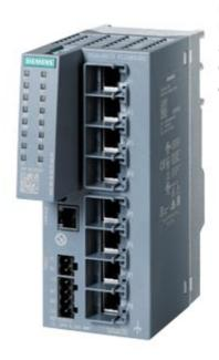
SCALANCE XC208G EEC Manageable layer 2 IE switch; 8x 10/100/1000 Mbit/s RJ45 ports; 1x console port; Diagnostics LED; Redundant power supply; with painted printed circuit boards; NAMUR NE21-compliant; Temp. range -40 °C to +70 °C Mounting: Standard mounting rail/S7 mounting rail/wall; Redundancy functions; Office features (RSTP, VLAN,...); PROFINET IO device; Ethernet/IPcompliant; C-PLUG slot;
