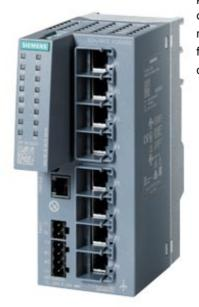
SCALANCE XC208EEC Manageable layer 2 IE switch; 8x 10/100 Mbit/s RJ45 ports; 1x console port; Diagnostics LED; Redundant power supply; with painted printed circuit boards; NAMUR NE21compliant; Temp. range -40 °C to +70 °C Mounting: Standard mounting rail/S7 mounting rail/wall; Redundancy functions; Office; features (RSTP, VLAN,...); PROFINET IO device; Ethernet/IPcompliant; C-PLUG slot;
