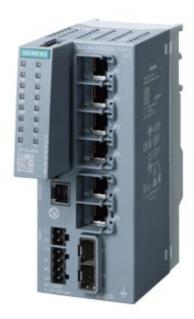
SCALANCE XC206-2SFP G EEC managed Layer 2 IE switch; IEC 62443-4-2 certified; 6x 10/100/1000 Mbps RJ45 ports; 2x 1000 Mbps SFP; 1x console port; diagnostics LED; redundant power supply; with painted printed circuit boards NAMUR NE21-compliant; temp. range -40 °C to +70 °C; mounting: DIN rail/S7 mounting rail/wall; redundancy functions; Office features (RSTP, VLAN,...); PROFINET IO device; Ethernet/IP-compliant; C-plug slot;
