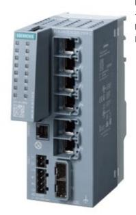
SCALANCE XC206-2SFP G Manageable layer 2 IE switch; 6x 10/100/1000 Mbit/s RJ45 ports; 2x 1000 Mbit/s SFP; 1x console port; Diagnostics LED; Redundant power supply; Temp. range -40 °C to +70 °C Mounting: Standard mounting rail/S7 mounting rail/wall; Redundancy functions; Office features (RSTP, VLAN,...); PROFINET IO device; Ethernet/IP-compliant; C-PLUG slot;
